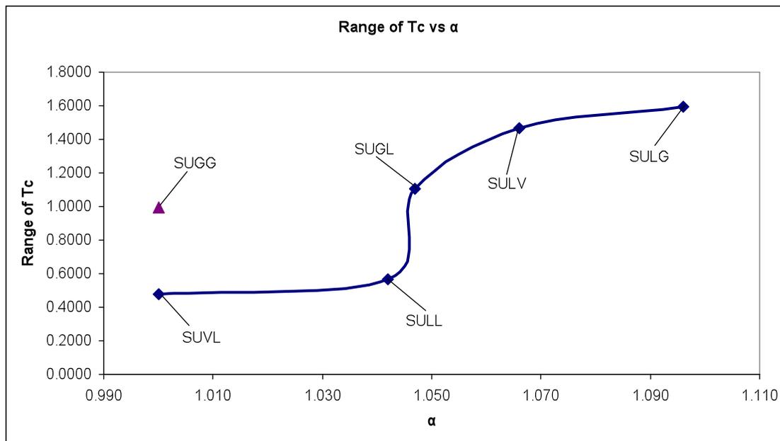
Figure 7. Graph showing the trend of increasing selectivity ( $\alpha$ ) relating to an increased range in correlation times for 1,1'-binaphthyl-2,2'-diyl hydrogen phosphate (BNP) analyte bound to each polymer, sodium undecyl (glycine, leucine or valine).
