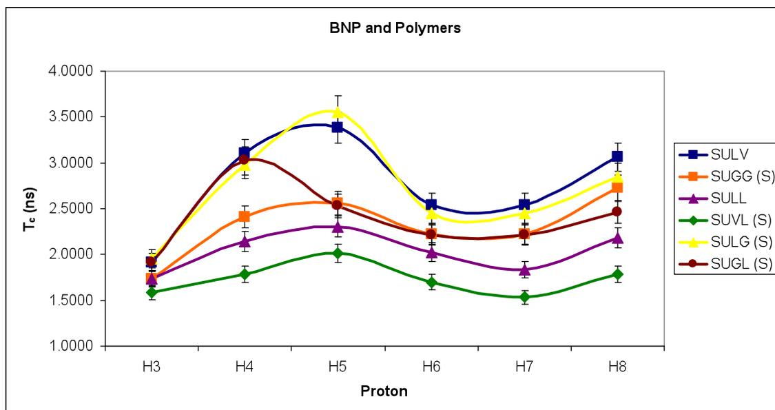
Figure 6. Correlation times of each proton for the six polymer micelles studied, sodium undecyl (glycine, leucine or valine). The polymers with the greatest amount of variation in their correlations times also have the most anisotropic movements.
