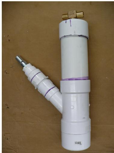
*Figure [3.1.3]: Fluidizing chamber*
