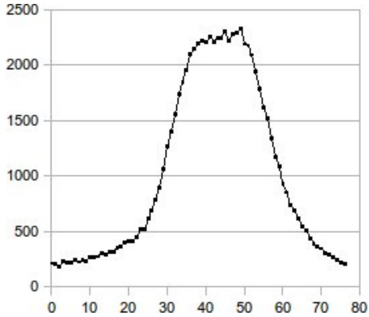
Figure 9: Hg 5460.74 with the slit positioned left of center. Notice the flat top of the peak and the bigger half-width, 60 second exposure
