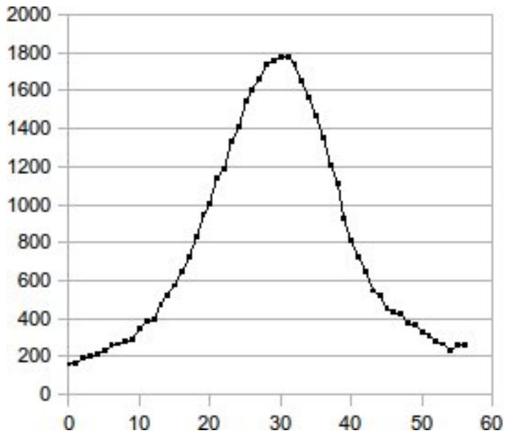
Figure 5: Hg 5460.74 with no left asymmetry after light shield is installed, 15 second exposure
