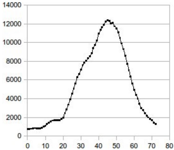
Figure 4: Hg 5460.74 with left asymmetry due to ambient light scatter, 100 second exposure
