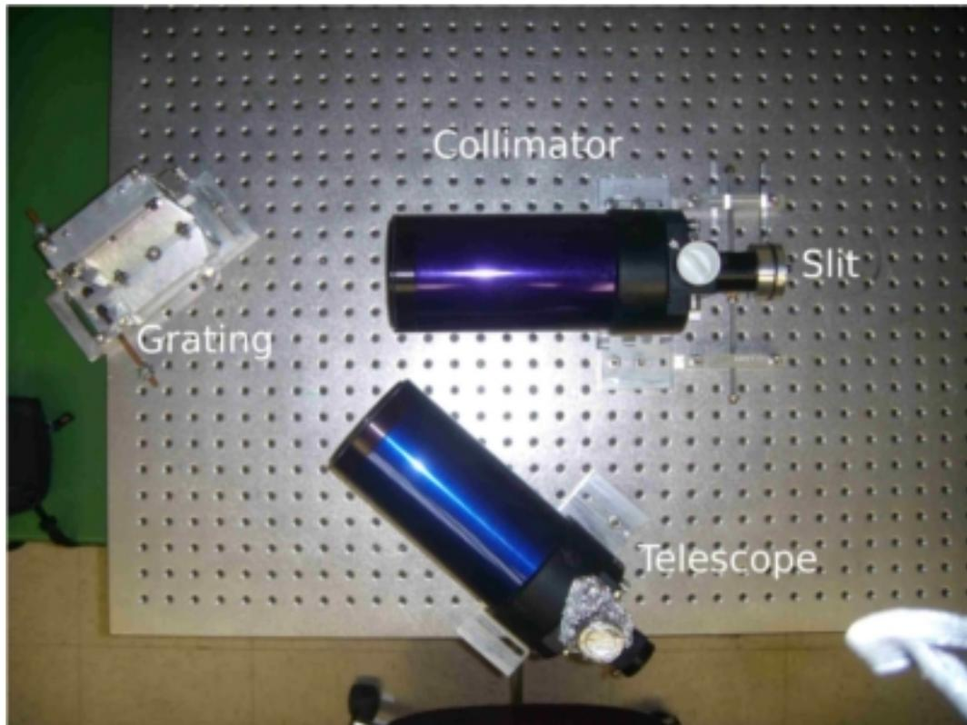
Figure 1: Basic grating spectrograph setup with a slit, a collimator, a reflection grating, and a telescope
