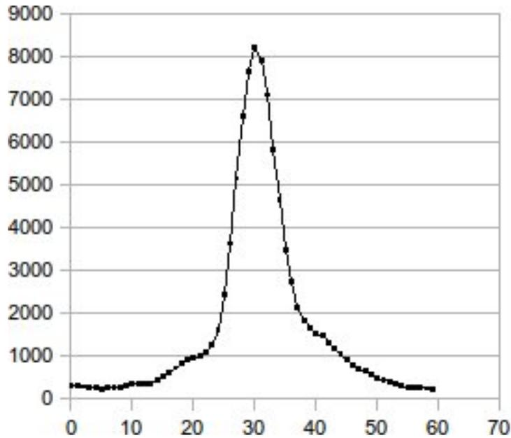
Figure 11: Final focused image of Hg 5460.74. Notice the asymmetry that remains on the right, half-width of 4 pixels, 100 second exposure
