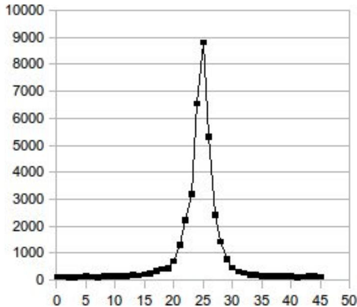
Figure 2: Hg 5460.74 without a Barlow lens, 100 second exposure
