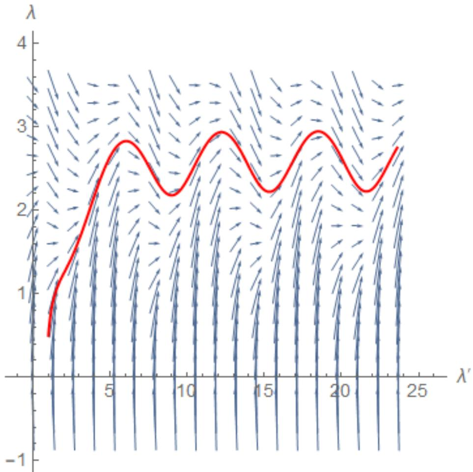
Figure 5: This solution depicts the case where the bias current is greater than the critical current. This produces a periodic solution. The voltage value that the oscillations are about depends on the value of the ratio relative to the voltage across the junction. The greater the ratio, the larger the value that the voltage oscillates around.
