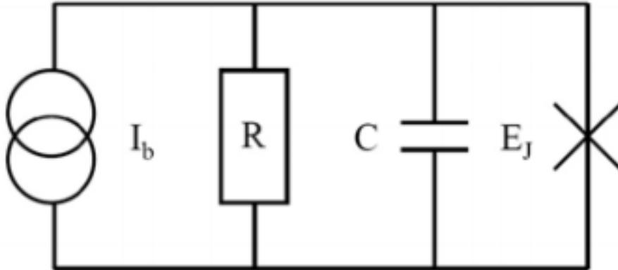
Figure 2: In the circuit, the Josephson junction is represented by the X, the resistor by the rectangle, the capacitor by the separated parallel lines and the current applied to the circuit is represented by the intersecting circles. In this circuit, both regular current and tunneling current can travel and to model this, it is use full to analyze this circuit using Kirchhoff's voltage and current laws. This figure was obtained from [3].
