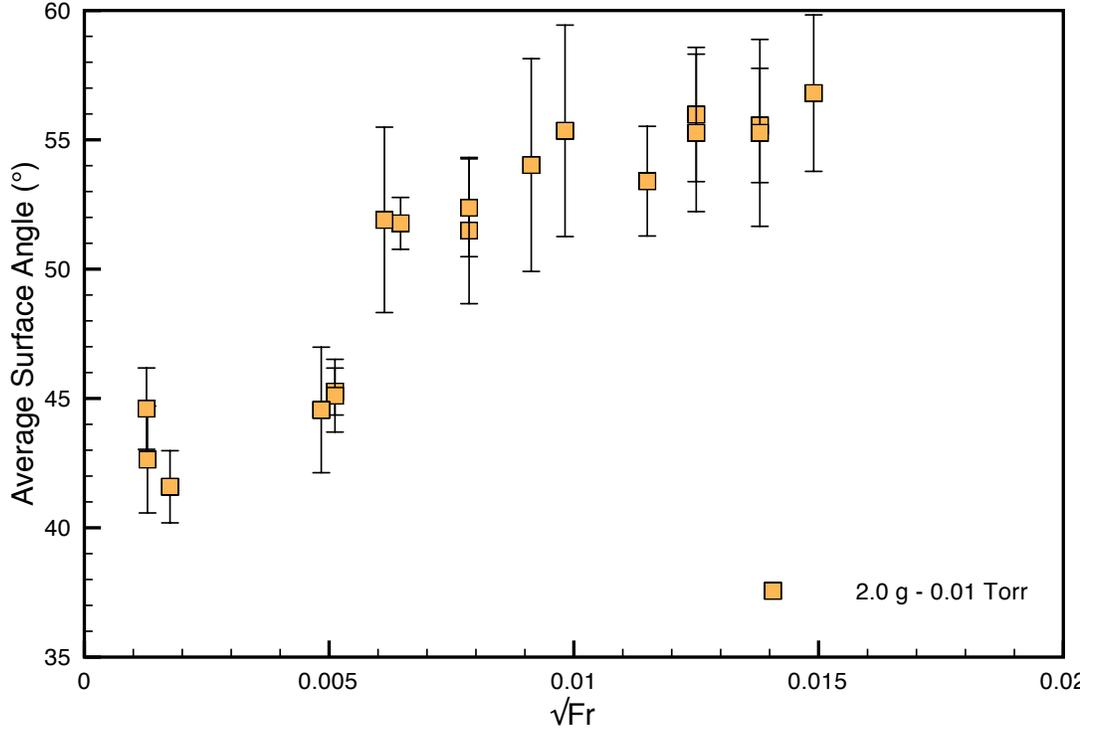
Figure 10: Measured surface angles for OB-1. Error bars indicate the upper and lower bounds of the measured angles. The top horizontal bars denote the average  $\beta$  measurements and the lower horizontal bars denote the average  $\alpha$  measurement in each measurement set..
