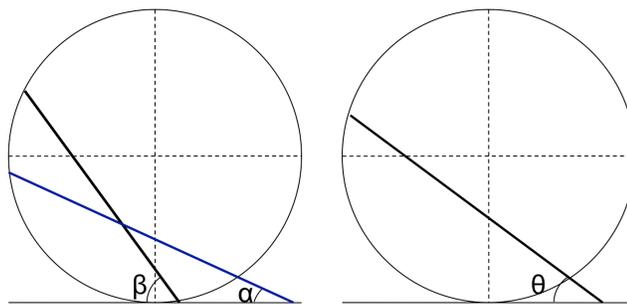
Figure 7: Surface angle regimes for lunar *mare* simulants. In the first regime, the simulant will build up to the maximum angle of stability  $\beta$  before collapsing to  $\alpha$ , the relaxation static angle. In the second regime, the transition occurs so rapidly, the simulant maintains a constant flowing surface designated by  $\theta$ .
