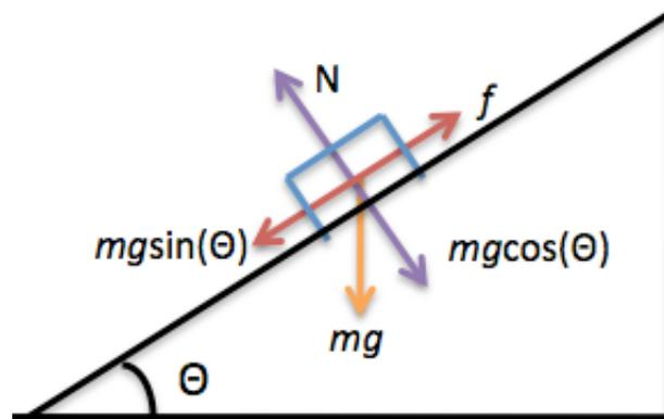
Figure 2: Forces on a mass resting on an inclined plane. A body of mass (in this instance, a granular particle) will experience forces due to gravity, friction and the normal force.
