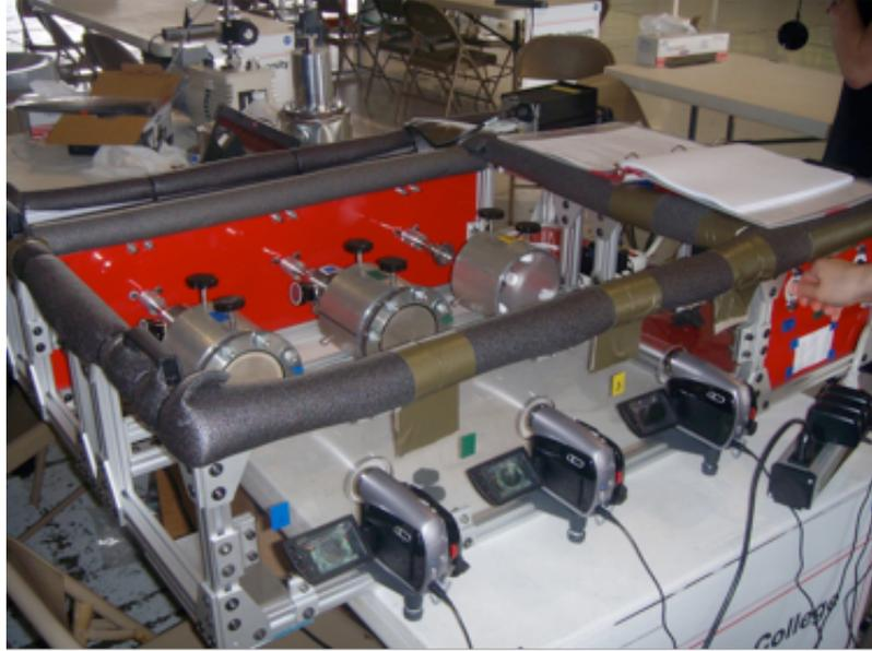
Figure 6: Experimental Rig. Each drum is loaded with one cup of lunar simulant, GRC-3 and JSC-1A in this particular image. Three miniDV cameras record the repose behavior for later analysis. Note the vacuum fittings for low pressure trials.
