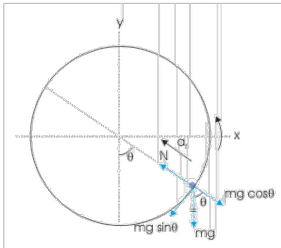
Figure 4: A force diagram of a mass in a rotating cylinder. Image Credit: Sunil Singh.
