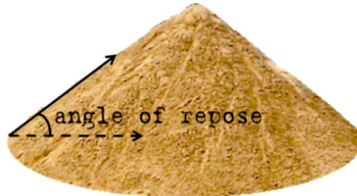
Figure 1: Static Angle of Repose.
