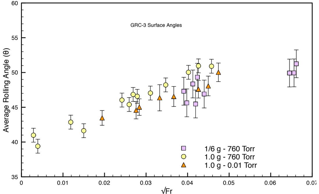
Figure 9: Measured surface angles for GRC-3. Error bars indicate the upper and lower bounds of the measured angles. The top horizontal bars denote the average  $\beta$  measurements and the lower horizontal bars denote the average  $\alpha$  measurement in each measurement set..
