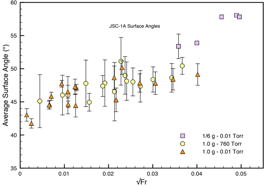
Figure 8: Measured surface angles for JSC-1A. Error bars indicate the upper and lower bounds of the measured angles. The top horizontal bars denote the average  $\beta$  measurements and the lower horizontal bars denote the average  $\alpha$  measurement in each measurement set. Uncertainty for most lunar (1/6-g) data is not available because each data point represents only one or two angle measurements.
