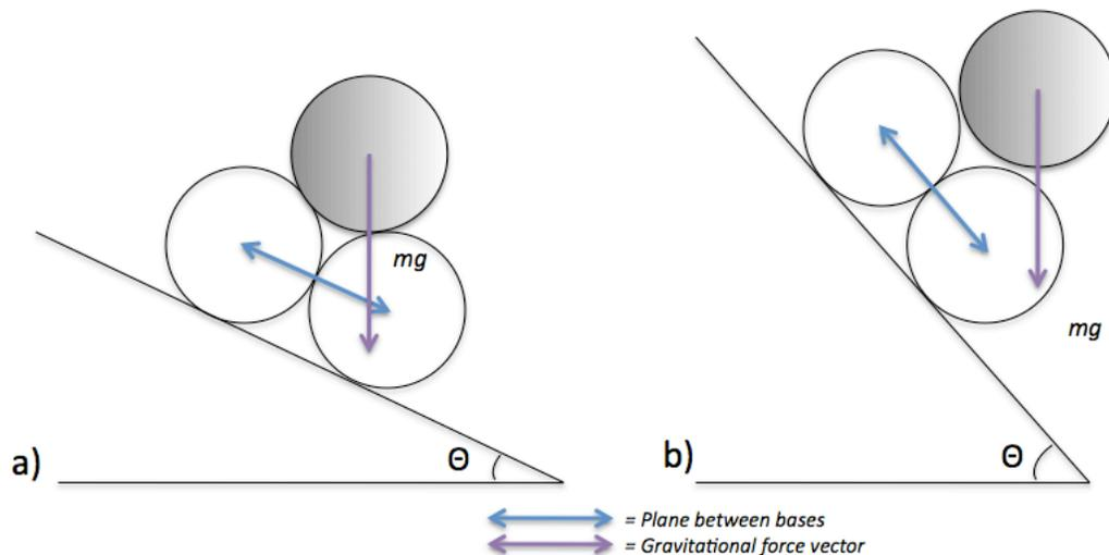
Figure 3: (a) The top spherical particle is stable so long as the gravitational force vector points through the plane created between the center points of the base spheres. (b) An unstable configuration,  $\theta$  is greater than the maximum angle of stability,  $\theta_m$ .
