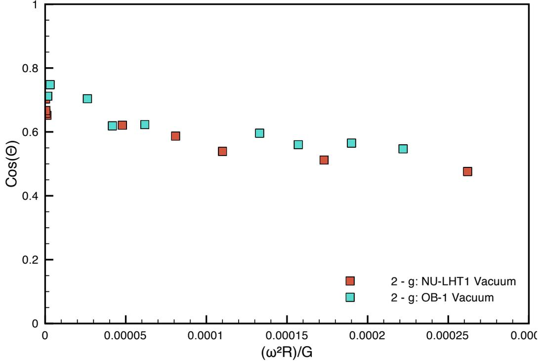
Figure 12: Measured surface angles for NU-LHT1 and OB-1. Plot of  $\cos(\theta)$  to  $\frac{\omega^2 R}{g_{eff}}$ . No error bars are included in this graph but each angle measurement has uncertainties, much like in the previous graphs.
