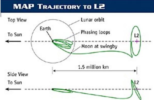
Figure 5: Here is an illustration of the path WMAP had to take to get to L2. [7].
