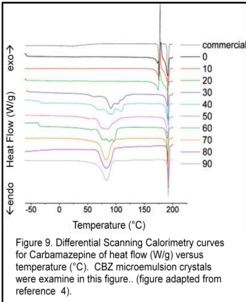
being given off (exothermic). In figure 9, the top line represents the commercial Carbamazepine. The first peak seen was at 175°C. This downward peak represented a taking in of heat (endothermic) and was the melting of the commercial P-monoclinic form ( $\beta$  CBZ) (figure 10). The next peak seen in figure 1 was at 178°C and
