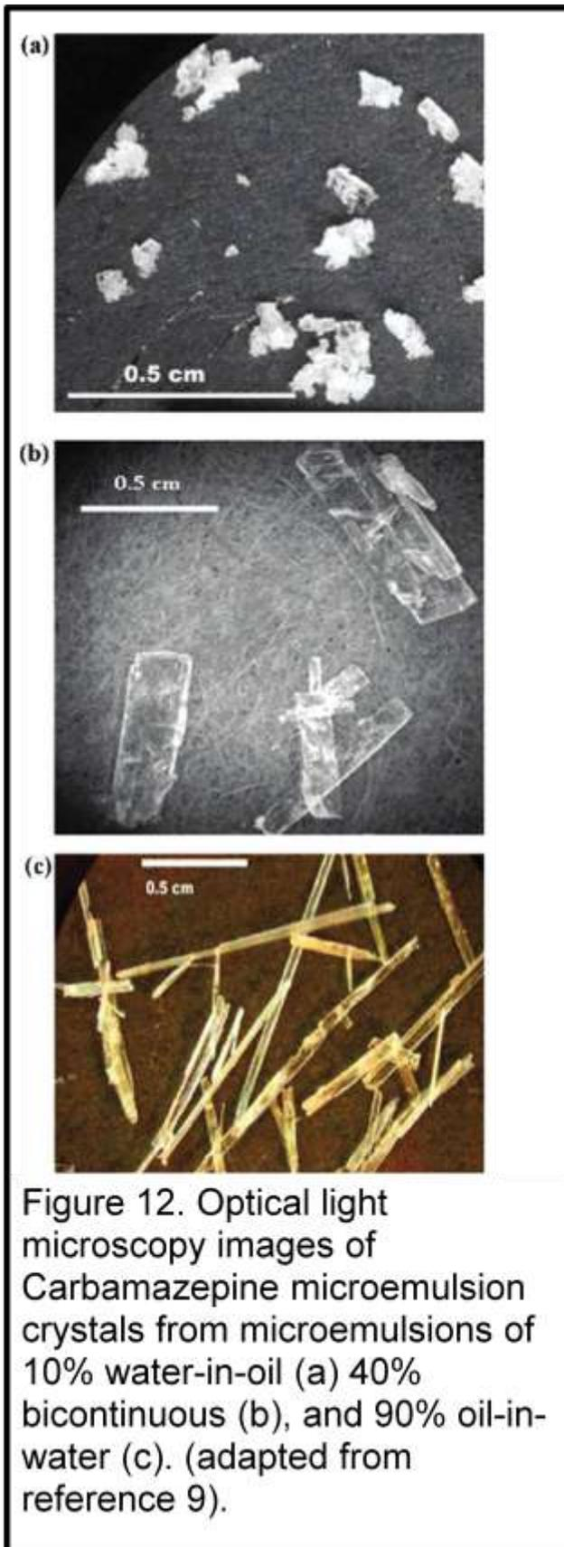
Optical light microscopy was used to get a closer look at the surface of the microemulsion crystals in order to more closely observe the crystals surface structure (figure 12; a-c). Figure 12a represents the 10% W/O microemulsion crystal. This microemulsion crystal had prism-like structures that measured 2 to 4 millimeters in width and 3-5 millimeters in length. These prism-like microemulsion crystals were formed in a test tube at room temperature (25°C) after 3 weeks without agitation.
