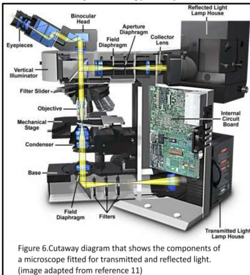
must reflect off of the surface back to the microscope.<sup>11</sup> Reflected Light Microscopes typically have two eyepieces and a trinocular tube head where a digital camera is often mounted in order to take pictures of the crystals surface.<sup>11</sup> The stage of the microscope is controlled electronically with a specimen holder which allows for precise movements and better focusing.<sup>11</sup> Light starts in the lamp
