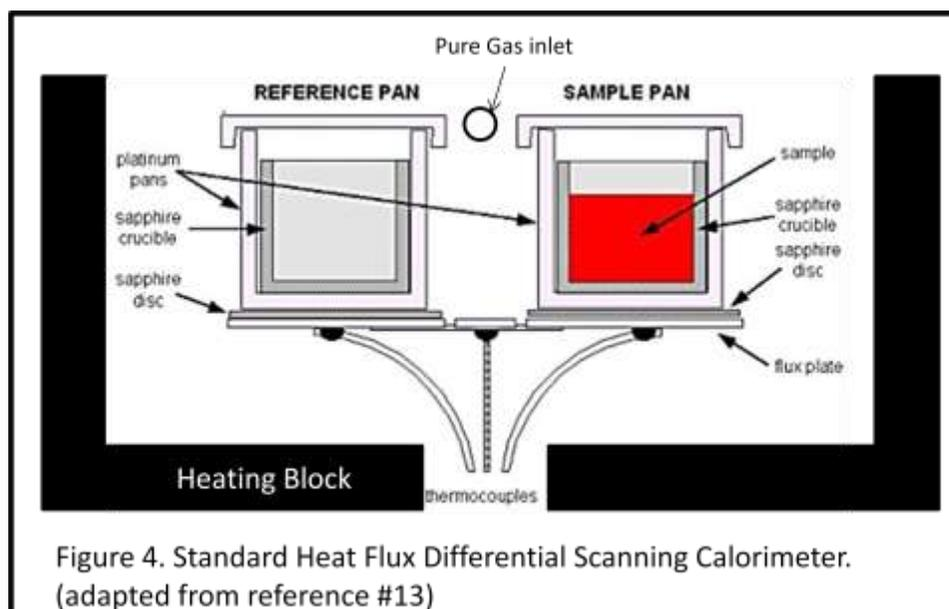
microemulsions.<sup>9</sup> Heat flux DSC measures the differences in the heat flow between a sample crystal and a reference crystal.<sup>9</sup> A reference crystal is used to see what is expected and what is obtained from the new sample. The crystals
