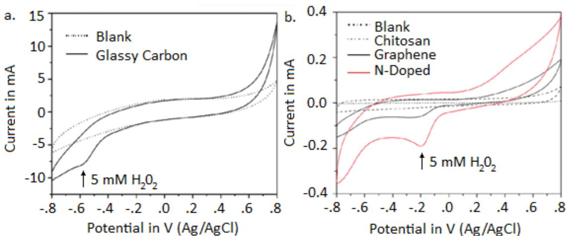
Figure 12. Cyclic voltammograms of a glassy carbon electrode in the presence and absence (Blank) of 5 mM hydrogen peroxide (a). Cyclic voltammograms of 5 mM hydrogen peroxide using a chitosan electrode, a graphene electrode and a nitrogen-doped graphene electrode (b)
