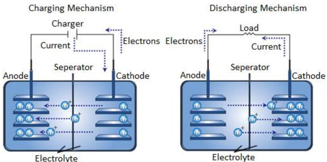
Figure 1. Charge and Discharge mechanisms of a lithium ion battery<sup>1</sup>
