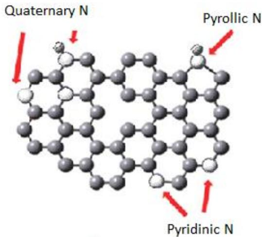
Scheme 1. A ball and stick model representing the lattice structure of nitrogen-doped graphene. Gray atoms represent carbon, while white atoms represent nitrogen and striped atoms represent hydrogen. A sample defect is displayed in the center of the diagram.
