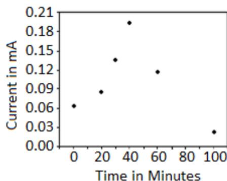
Figure 11. A plot of the cyclic voltammetric signal of 5 mM  $H_2O_2$  versus plasma exposure time of the graphene coated glassy carbon electrode. Time 0 indicates no plasma treatment
