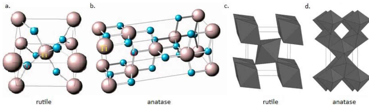
Figure 6. Structure of titanium dioxide presented as unite cells of rutile (a) and anatase (b) polymorphs as well as edge-sharing  $\text{TiO}_6$  octahedral diagrams of rutile (c) and anatase (d) crystals
