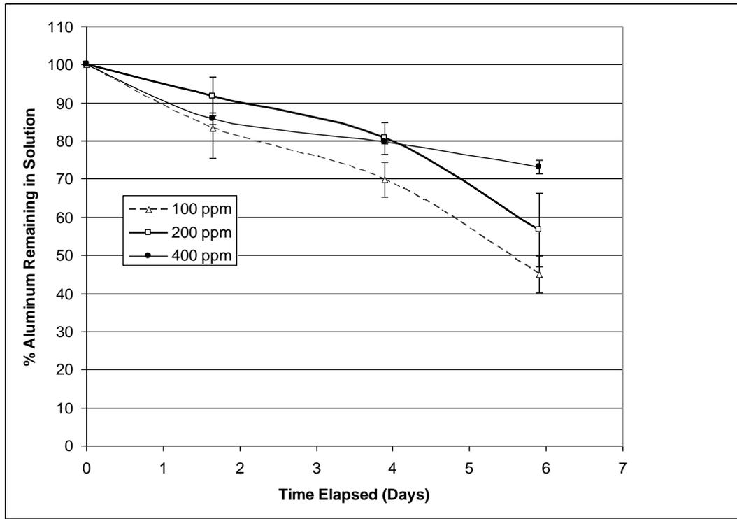
**Figure 3:** % of the original aluminum remaining in treatment solutions at a given time. Points on the graph represent odd-numbered sampling periods. Error bars represent SD (n=3)
