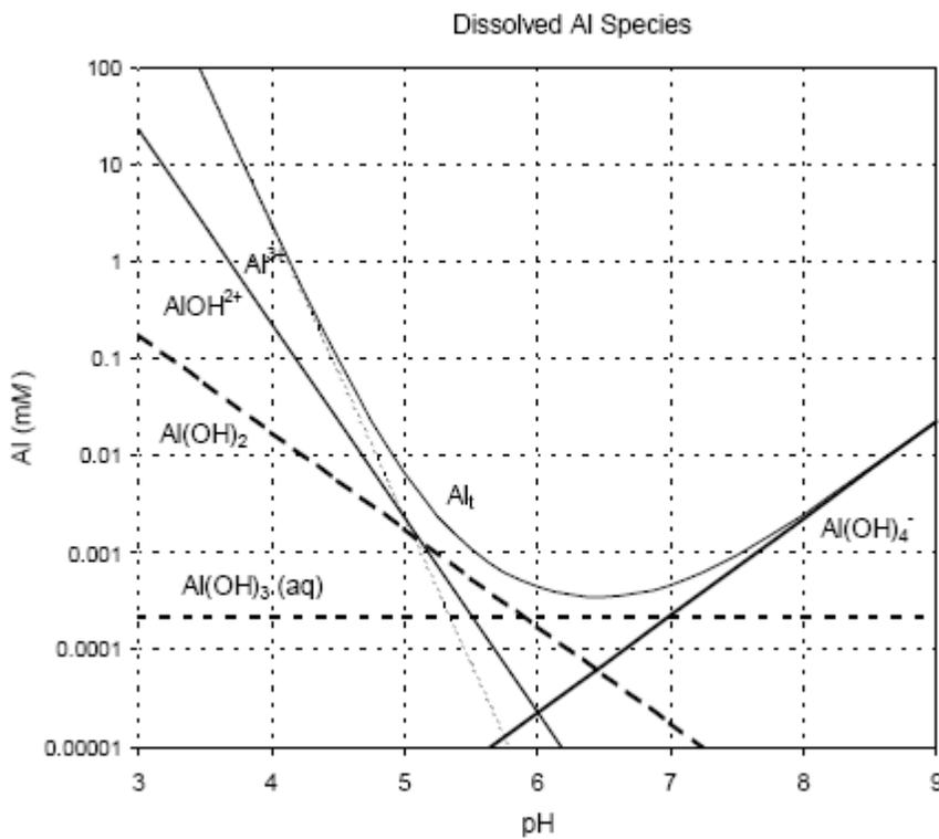
**Figure 4 (Left).** Solubility of aluminum species (and total aluminum,  $Al_t$ ) in relation to pH in a system in equilibrium with microcrystalline gibbsite (0.001 mM = 0.027 mg/L). (Source: Environment Canada, 2000).
