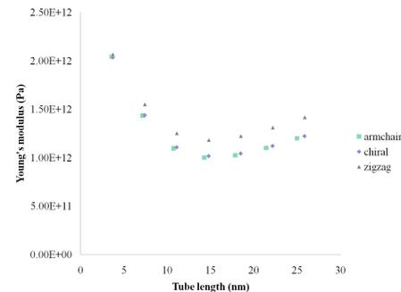
Young's moduli for three CNTs at variable lengths. The finite sized scaling analysis concludes that data from CNTs which are shorter than 14 nm are unreliable.
