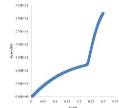
The estimated stress-strain curve of a zigzag SWCNT. Strains greater than .04 are considered outside the linear regime.
